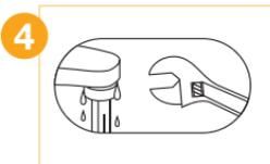
**4.** Turn on the water. If the aerator leaks, use the wrench to tighten until snug. Use a cloth to protect the finish. **DO NOT OVER-TIGHTEN.**
