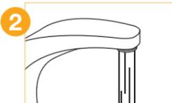
1. Remove the old aerator from the faucet. Use a wrench if needed. Use a cloth to protect the finish.
