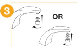
3. **TURN OFF WATER.** Screw on the new aerator and hand-tighten.
